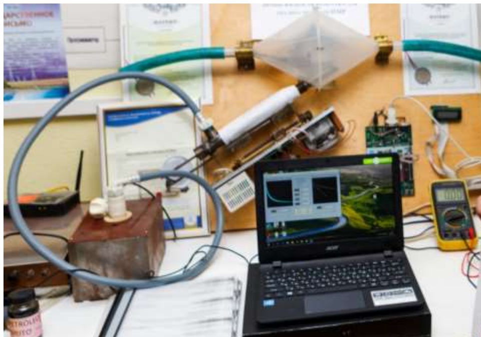
Fig.1. Testing ground (stand) for studying of on-line probe sampling system and analysis of oil samples by PMRA-II.
