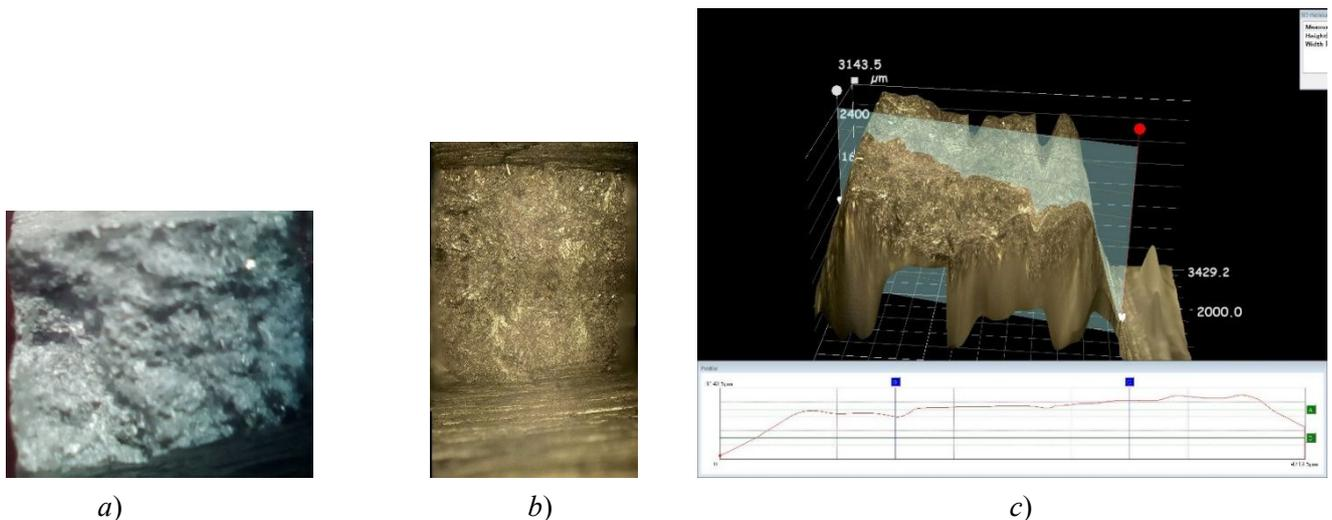
Fig. 1. The fracture surface of the sample: *a* – the optical macrostructure x40; *b* - macrostructure in Optimal Image mode; *c* – 3D structure with profilograms on the highlighted section
