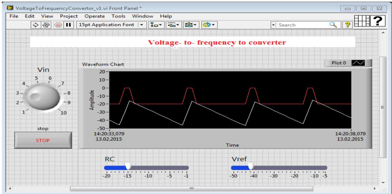
Figure1 Interface of laboratory stand
