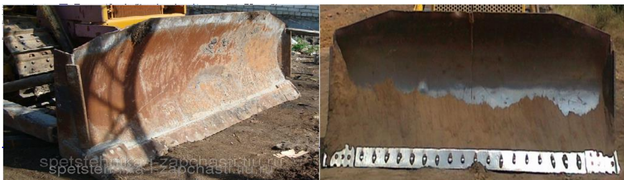
Figure 1 - Rust and adhered soil
