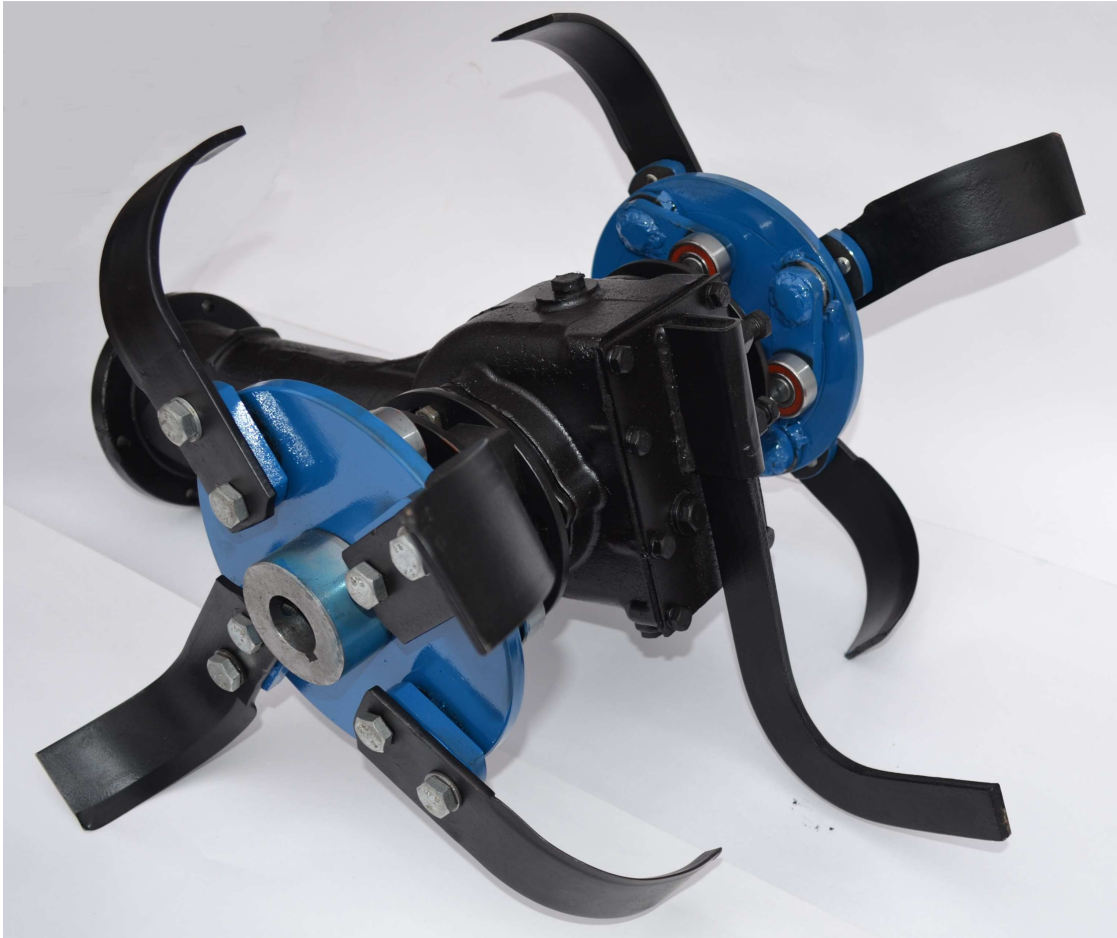
Picture 6 – a pilot model of working element with the constant cutting angle
